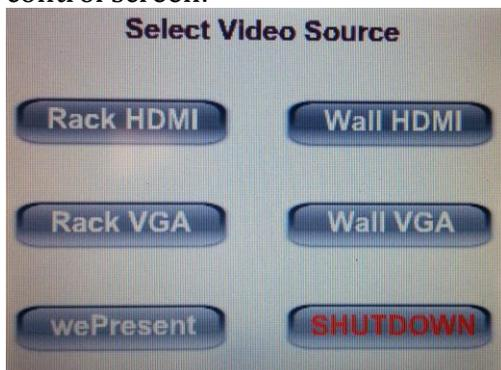
Press the button for the input you wish to use. If you're using VGA and want to play sound, you'll need to connect the audio cable attached to the VGA cable to the headphone jack on your computer. If you're using HDMI, your computer's audio should automatically play through the HDMI cable. If not, you'll need to set that up on your computer.
